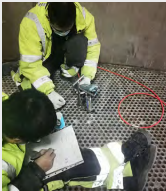
Reactor pressure test during catalyst loading in January 2021
