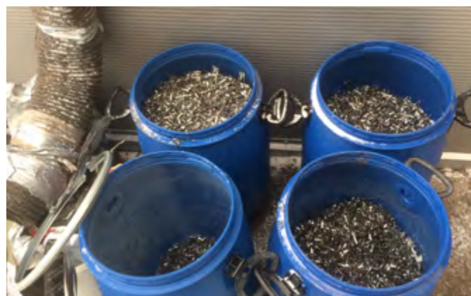
Collected damaged packing material
